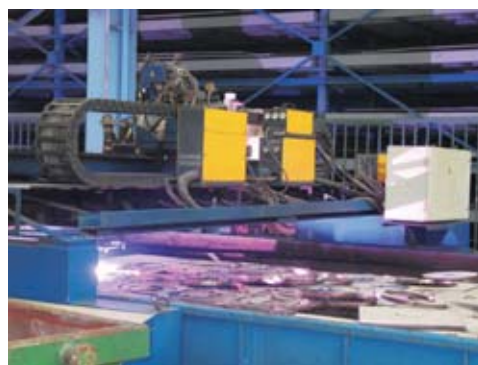
激光切割设备 Laser cutting equipment
